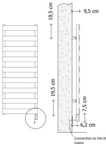
Connection to the electricity mains with Standard Edge
