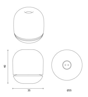
MATERIAL: STRUCTURAL RIGID POLYURETHANE WITH HIGH MECHANICAL STRENGTH.
